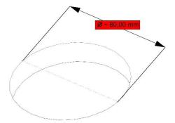
Hole for device mount is Ø 80mm
