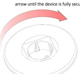
Rotating the upper cover of the device to the right, provides the access to built-in sockets. When the device is not in use, rotate it in opposite direction to close the device and so protect the modules from external influences.
