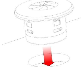
Rotate the bottom cover in the direction of the "FIX" arrow until the device is fully secured
