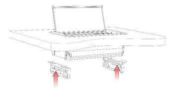
Put the fixators back on the device and push them strongly up to the plate of table. Connect the device to low voltage network with a cable.
