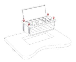
Position the device in an opening hole and gently descend until the flange unit grabs the board table.
