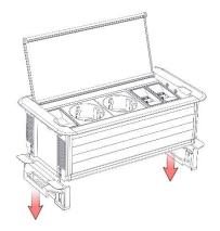
Remove fixators from the device by pulling them down.
