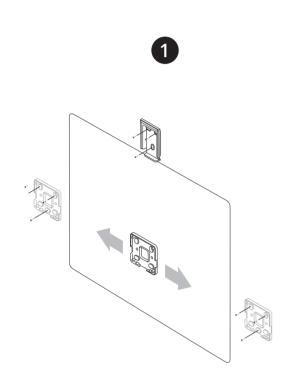
Install the rectangular Kaptivo mounting plate centered above board. Then install the square control pad mounting plate on your preferred side of the board. Use supplied screws. Maximum board size: 6 ft x 4 ft (1.8m x 1.2m).
