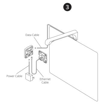
Wi-Fi Connection: Connect Kaptivo data cable and USB power cable to their respective sockets inside the control pad.
