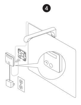
Push the control pad onto the mounting plate. Plug in the power adapter to outlet if power is not supplied by Ethernet connection.
