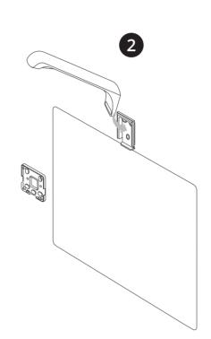
Slide Kaptivo unit onto mounting plate.
